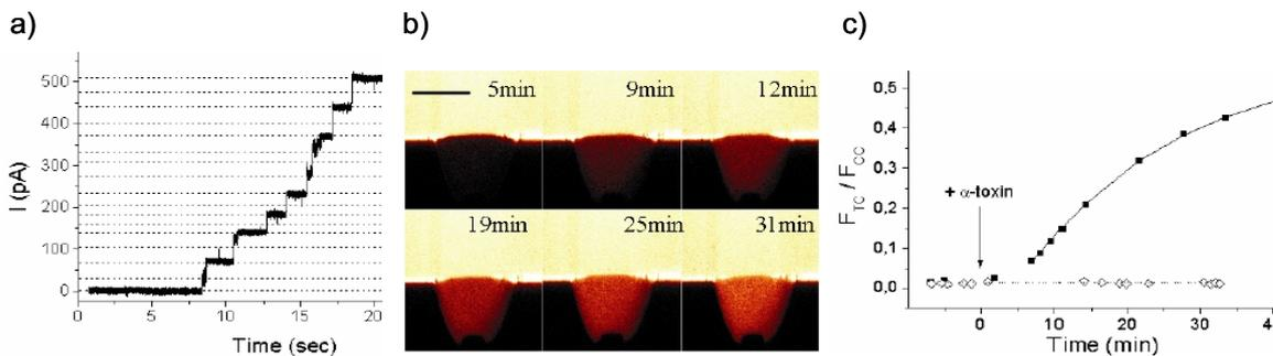
The formation of  $\alpha$ -hemolysin pores into a bilayer was recorded with single channel resolution (a). The transport of calcein, a water soluble dye with a Stokes diameter of about 0.65 nm was observed. An increase of brightness in a microcavity (z-scan) of about 70  $\mu$ m (depth) x 70  $\mu$ m (diameter) is detected after addition of  $\alpha$ -hemolysin (b,c).
