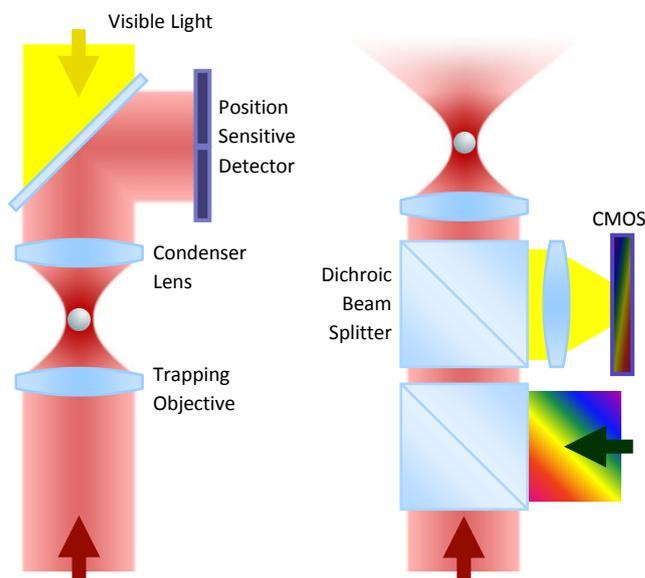
Left: The common principle of force measurement. Infrared laser light (red arrow) passing through the trapped particle (forward scattered light) is collected and projected onto a detector sensing the particle's deflection. The condenser in close proximity (ca. 1mm) to the trapping objective needs to be precisely adjusted. It significantly limits the experimental space and is susceptible against drift and misalignment.
